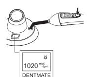
4. While holding the unit, press and release the ON-OFF Button. The radiometer will then provide a reading of the light intensity on the cradle display.
